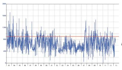
**Fig. 2** Mean monthly Electrical Conductivity at Singleton 1993 – 2013. Red line is the salinity target.
