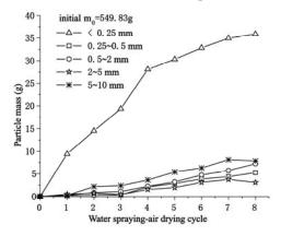
Fig. 4 Particles change in mass during water spraying-air drying cycles slaking test
