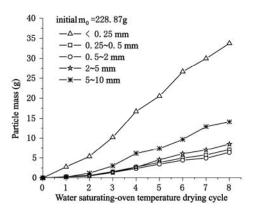
Fig. 5 Particles change in mass during water saturating-oven temperature drying cycles slaking test
