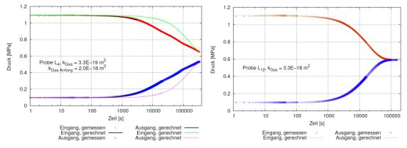
*Figure 4 Test results of core sample*  $L_4$  *and*  $L_{12}$
