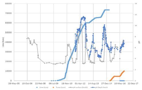
Figure 3 Lime and Trona addition, south surface and depth pH.
