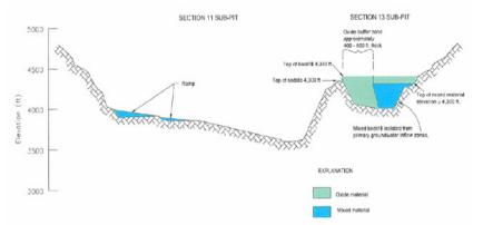
Figure 1 Cross-sectional schematic of Lone Tree pit and sub Section 13 backfill.
