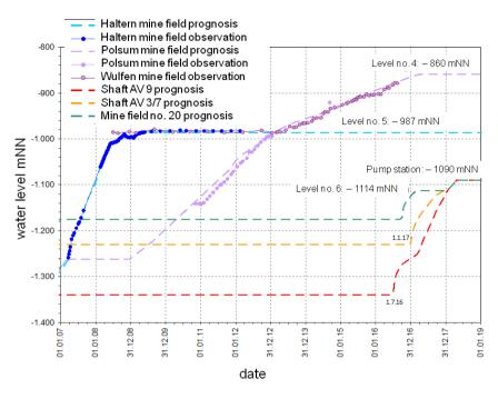
Figure 6 Simulation of exemplary mine water levels and monitoring results (DMT)
