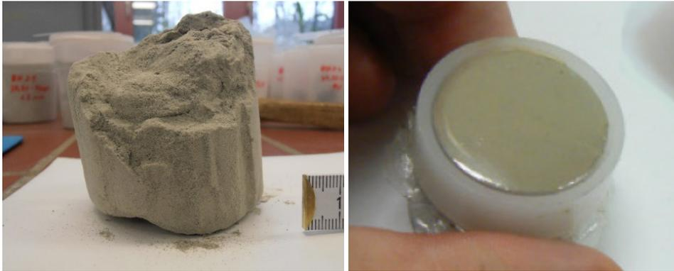
**Figure 3** left: drill core sample; right: cup with dried, homogenized tailing material
