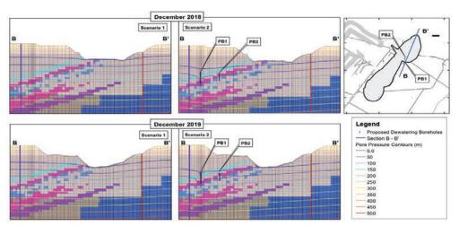
Figure 5 Section through Pit 2, PB1 and PB2 Showing Phreatic Surface and Pore Pressure – 2018 and 2019
