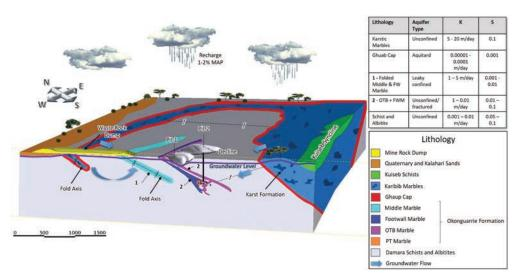
Figure 1 Conceptual hydrogeological model
