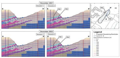
Figure 6 Section through Pit 2, PB1 and PB2 Showing Phreatic Surface and Pore Pressure - 2021 and 2023
