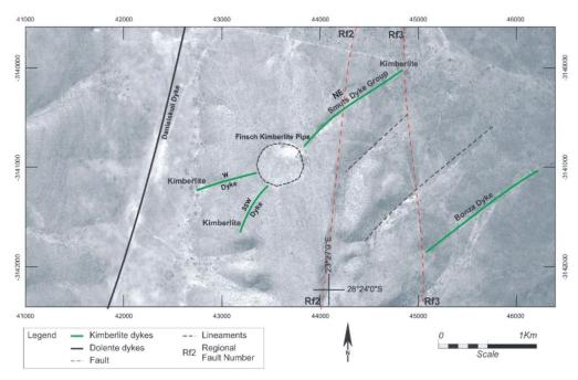
Figure 2 Aerial photograph of Finsch kimberlite pipe and kimberlite dykes (pre-cursors) pre- mining 1959
