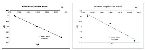
Figure 3 The Arrhenius plot for the adsorption of cadmium by (a) NT biochar and (b) PT biochar
