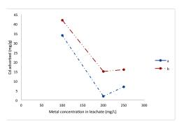
**Figure 4** Effect of whole solution concentration on the adsorption of Cd with (a) NT biochar and (b) PT biochar
