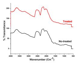
Figure 1 FTIR spectra of Non-treated and Pretreated biochars
