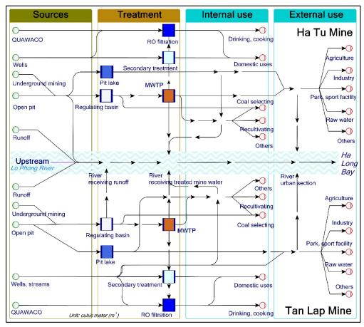
Figure 6 Material flow analysis of existing situation (Lo Phong Drainage Unit)
