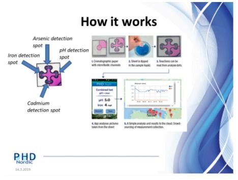
Picture 1 Monitoring concept setup (courtesy PHDNordic).
