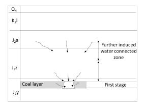
Figure 1 schematic map of hydrogeologic condition shifting at the Xiaojihan col mine
