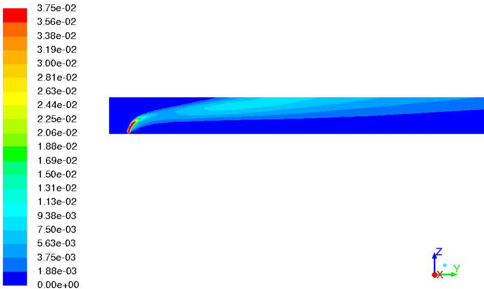
Figure 1 Pollutant concentration fields in vertical cross-section along the main stream. Diameter of outlet is 0.1 m. Concentration of the discharged brines is 375 g/L.
