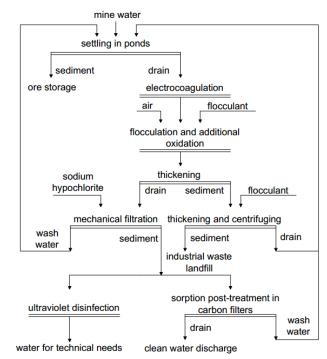
Figure Schematic diagram of mine water treatment
