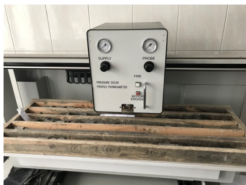
Photo 1. PDPK-400 permeameter A – profiling of permeability on rock cores; B – testing of individual rock samples
