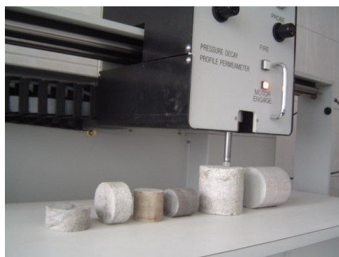
Photo 1. PDPK-400 permeameter A – profiling of permeability on rock cores; B – testing of individual rock samples
