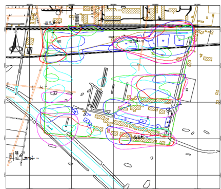
Fig. 7 Comprehensive results of the surface transient electromagnetic survey revealing water-rich anomalous areas
