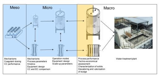
*Figure 2* Stages of process development and scale-up for the electrocoagulation of mining waters at meso. micro and macro levels, blue color – completed stages, yellow color – present stage.
