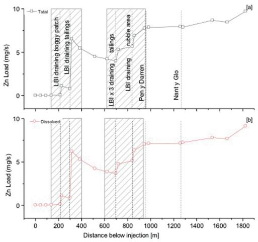
**Figure 4** Spatial profiles of total [a] and dissolved [b] instream Zn loads; total [c] Location of major inflows indicated with vertical dashed lines. Shaded areas = upper tailings ( $\approx$ 140-400 m) and lower tailings ( $\approx$ 620-950 m).
