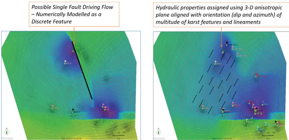
Figure 3 Example Hydrostratigraphic Zoning Methodologies Tested during Hazard Modelling Scenarios
