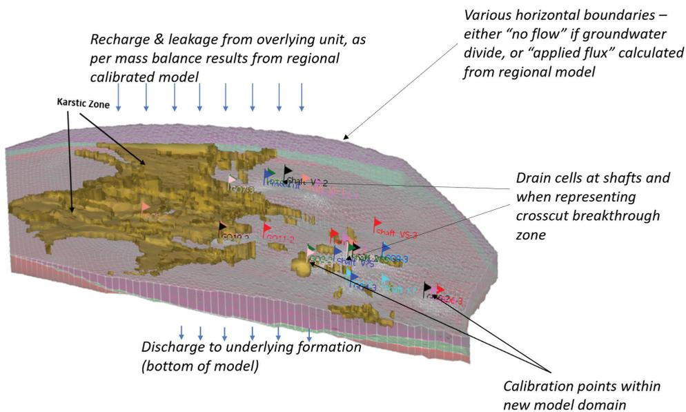
Figure 2 Example Boundary Conditions for Revised HGM Domain
