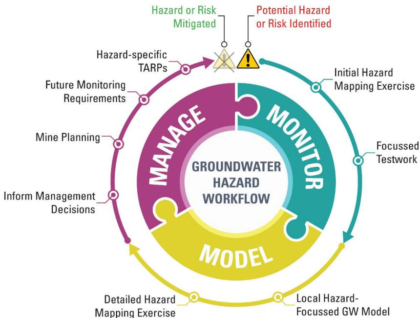
Figure 1 Groundwater Hazard Workflow
