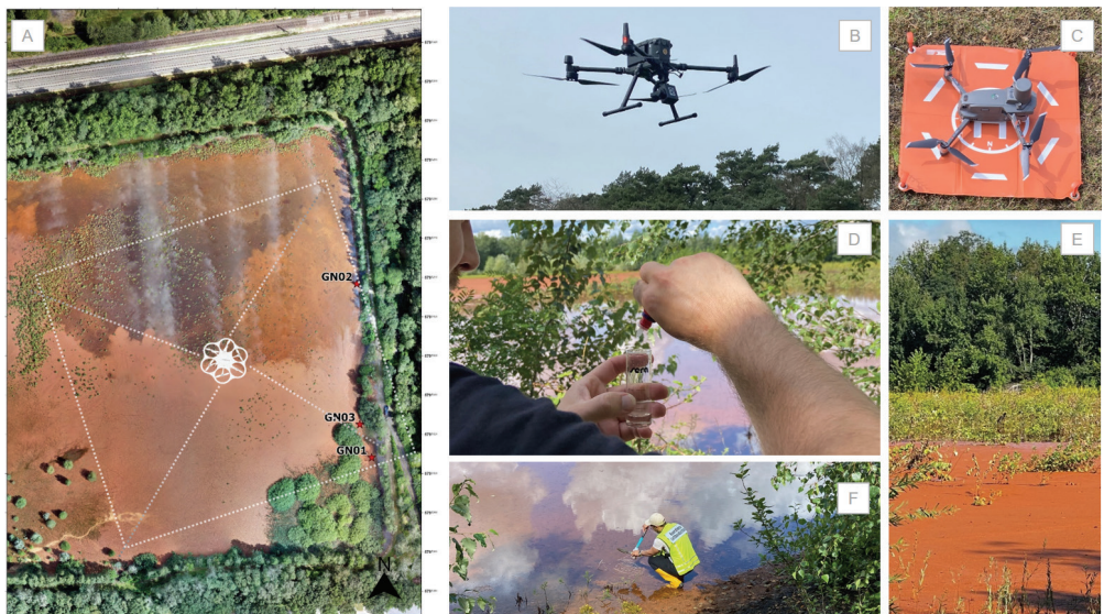
Figure 1 (a) Orthophoto of the Tailing facility at Ibbenbüren showing the UAS-borne hyperspectral scanned scene and sampling locations (red-starts). (b) Unmanned aerial system (BlackBird V2 Hyperspectral Sensor on board the DJI M300). (c) DJI Mavic 2 Enterprise Advanced Thermal drone. (d) Detail of in-situ Fe concentration measurement. (e) Detail of the area and the characteristic color of sewage sludge material. (f) Detail of field sampling acquisition (water and sediment)
