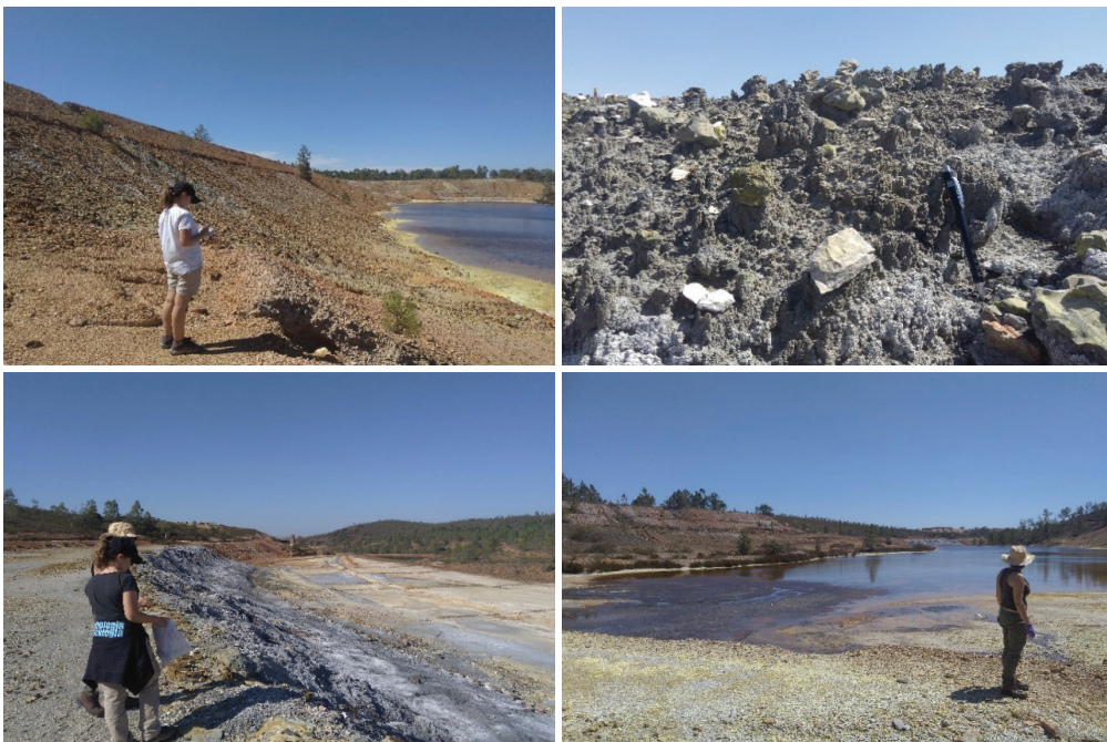
Figure 1 a) North view of landfill A1 highlighting the presence of saline efflorescences of sulfates (Al/Fe and Mg/Cu) at the landfill's base; b) General view of the A11 landfill composed predominantly of washed ore. Note the typical grey color with salt coverage; c) structures resulting from erosion in fairy chimneys; d) Abundance of sulfate blooms and filamentous acidophilic algae.
