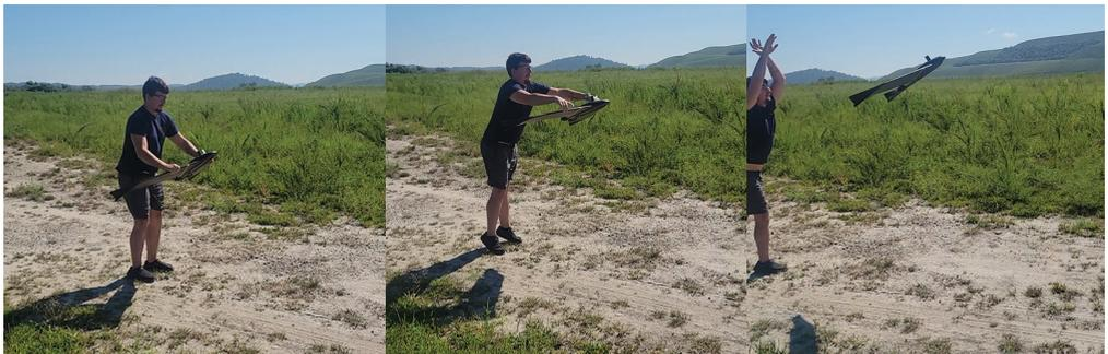
*Figure 1 Hand launch of eBee X fixed-wing UAV*
